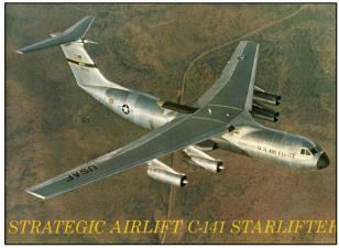
Capable of crossing any ocean nonstop at more than 500 miles per hour, the Starlifter could transport up to 68,500 pounds of payload, including 154 troops, 123 paratroopers, or a combination of troops and supplies. The C-141 replaced slower, piston-engined cargo planes in both strategic and tactical airlift missions, and it provided critical support to U.S. forces in Vietnam and Southwest Asia. The photo at left is from the cover page of Lockheed's C-141 Roll-Out Brochure.
