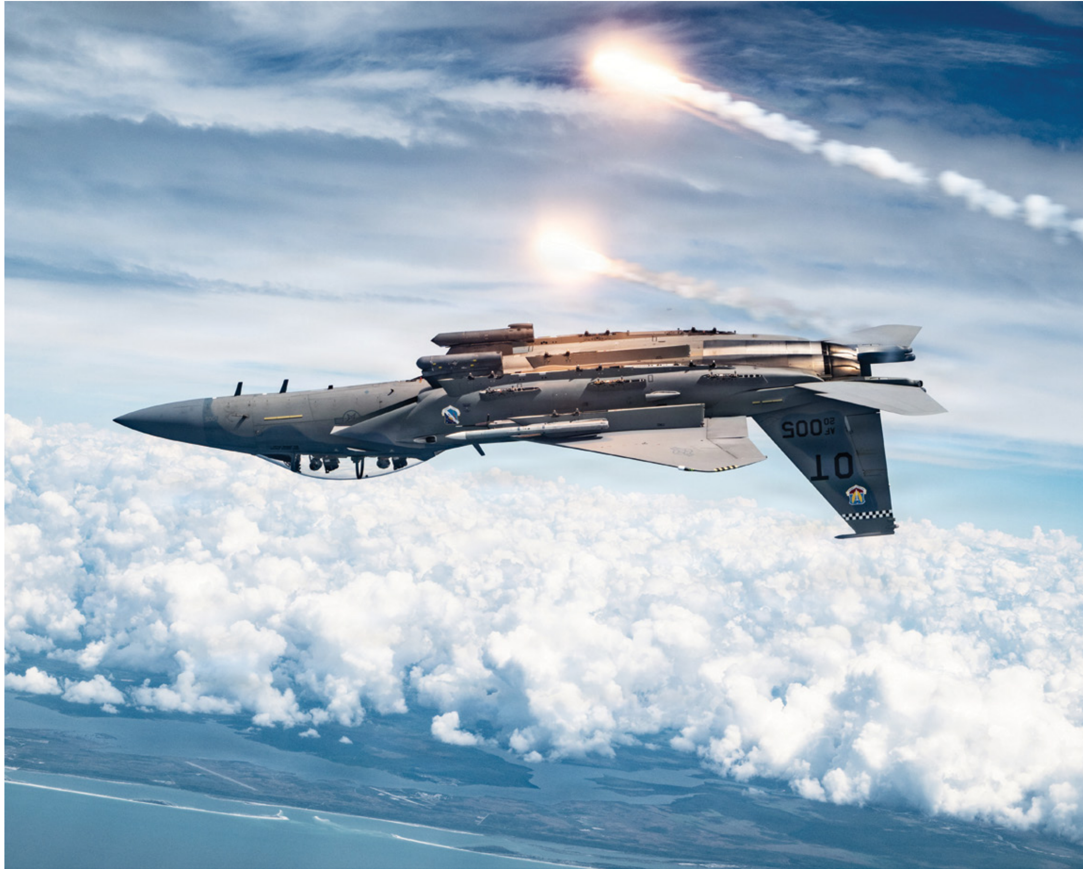
F lares deployed: An F-15EX Eagle II releases flares over the Gulf Coast, Fla., April 3, 2026. Flares act as infrared countermeasures designed to distract and defeat heat-seeking missiles by creating alternate heat sources away from the aircraft. Test wings continue evaluating next-generation survivability, radar and sensor capabilities. (U.S. Air Force photo by Tech Sgt. Thomas Barley) ▲
