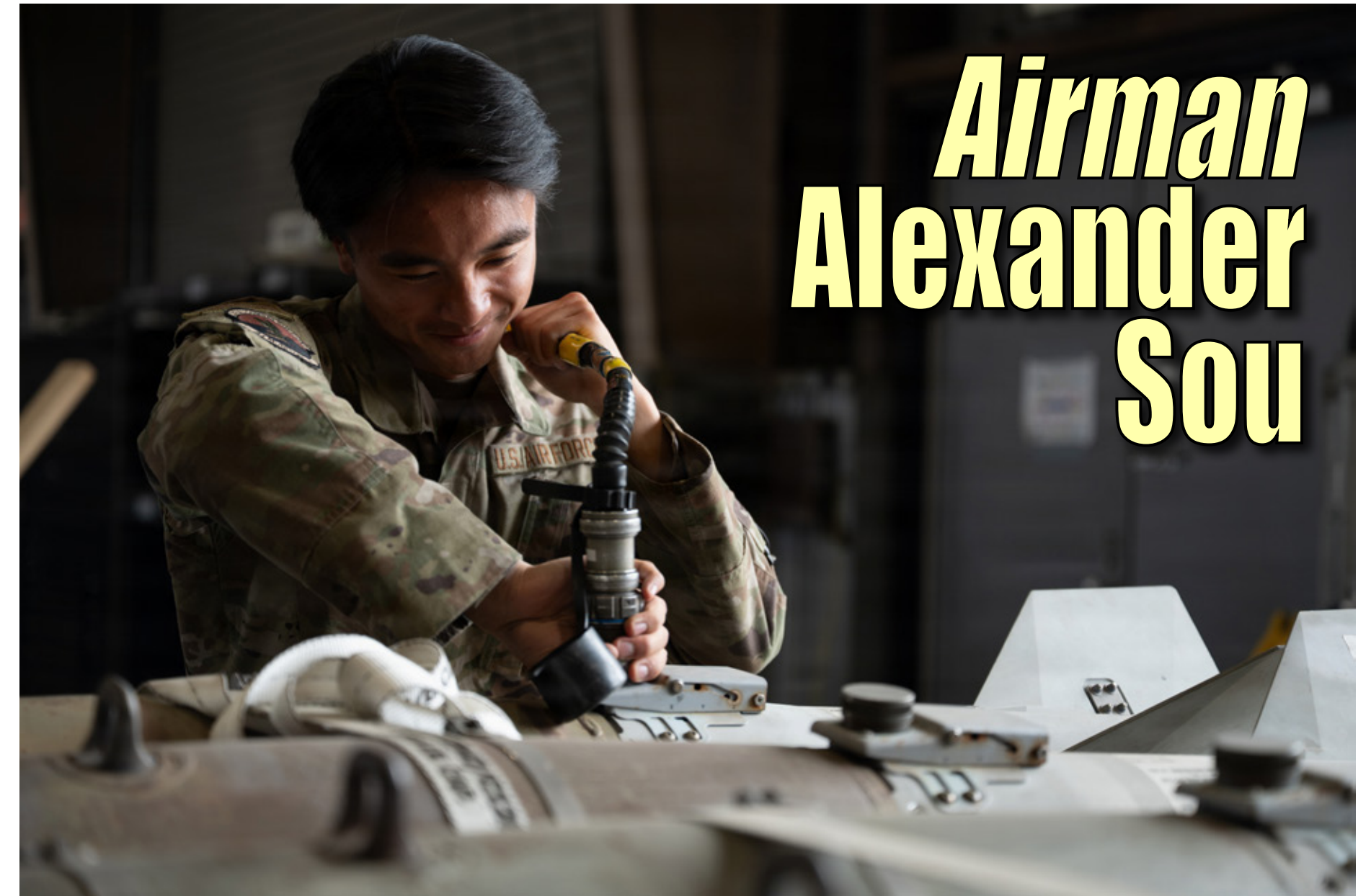
U.S. Air Force Airman Alexander Sou, 51st Munitions Squadron conventional maintenance technician, initiates built in testing of the tail kit at Osan Air Base, Republic of Korea, April 14, 2026. Sou's daily responsibilities include testing and maintaining munitions to utilize on F-16 Fighting Falcons. ▲
