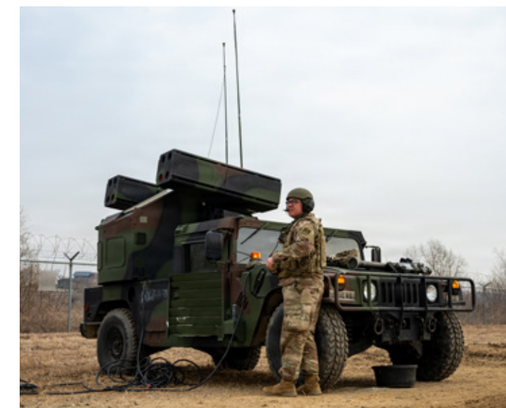
U.S. Army Staff Sgt. Pablo Chapa, Echo Battery, 6th Battalion, 52nd Air Defense Artillery Regiment air missile defense crew chief, searches for an unmanned aerial system during a joint training scenario as part of Freedom Shield 26 at Osan Air Base, Republic of Korea, March 11, 2026. The Avenger is a mobile air defense platform equipped with Stinger missiles designed to counter low-altitude threats, such as drones and aircraft. ▲
