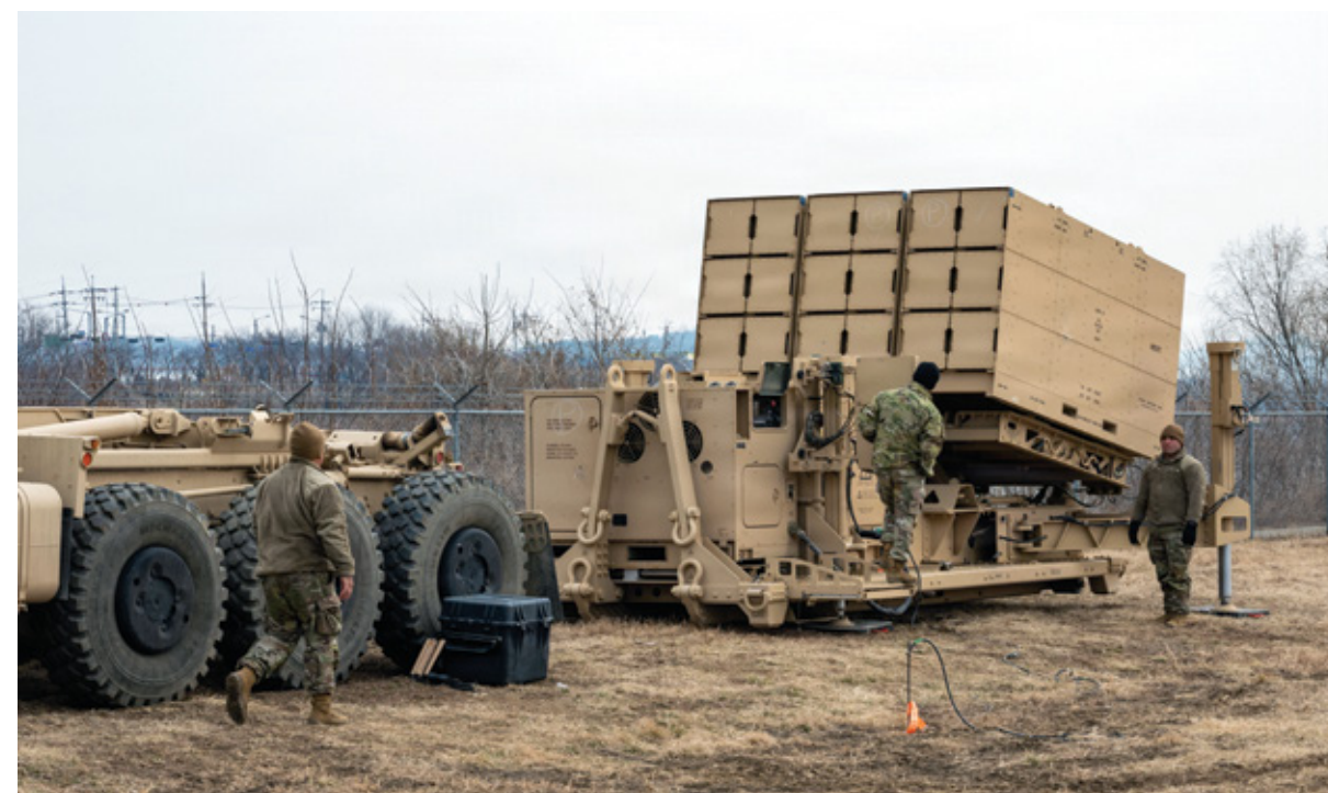
U.S. Army Soldiers inspect an Integrated Fires Protection Capability Increment 2 launcher during a joint training scenario as part of Freedom Shield 26 at Osan Air Base, Republic of Korea, March 11, 2026. IFPC launchers are mobile, ground-based weapon systems designed to defeat subsonic cruise missiles, groups 2 and 3 unmanned aircraft systems and other aerial threats. ▲
