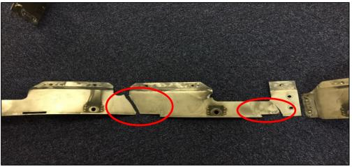
Figure 10: Fractures emanating from bracket wear (Tab Z-9)
