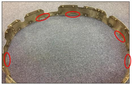
Figure 8: Turbine frame fairing wear marks (Tab Z-13)
