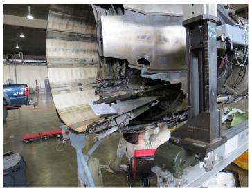
Figure 15: Exhaust nozzle burn damage from 3:00 to 6:00 (Tab CC-73)
