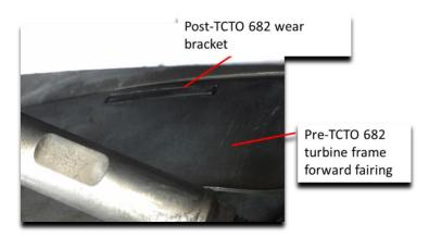
Figure 12: Forward fairing wear bracket worn through fairing (Tab CC-79)
