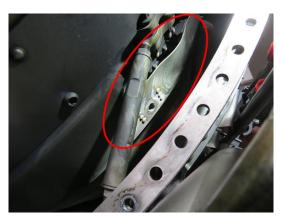
Figure 5: Turbine frame forward fairing with missing bolt at 4:30 position (Tab CC-75)
