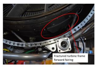
Figure 6: Turbine frame forward fairing damage at 5:30 position (Tab CC-75)
