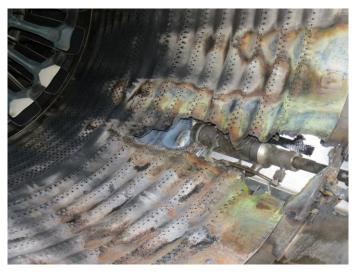
Figure 16: Burn-through on exhaust duct liner and duct at 4:30 (Tab CC-74)
