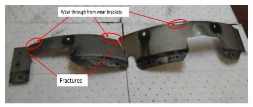
Figure 9: Fractures emanating from bracket wear (Tab CC-76)
