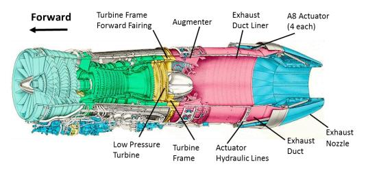
Figure 4: F110-129 Engine Schematic (Tab CC-63)
