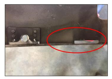
Figure 13: Forward fairing wear bracket worn through fairing (Tab Z-8)
