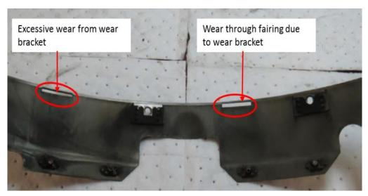
Figure 7: Turbine frame fairing wear marks (Tab CC-76)
