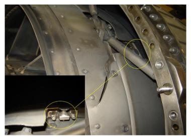
Figure 17: Fairing failure in 2009 event (Tab CC-77)
